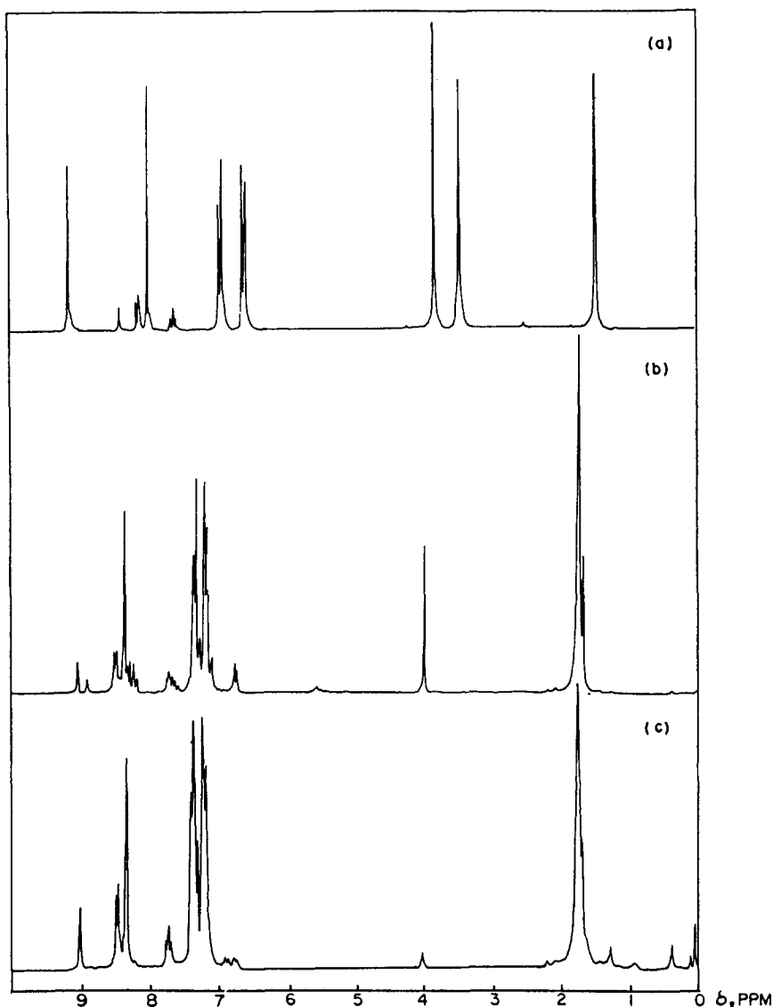
Figure 2 ^1\text{H-NMR} spectra of (a) initial mixture (BPA + DMI + DMT) in dimethyl- d_6 sulfoxide, (b) prepolymer A in \text{CDCl}_3 , and (c) crude final polyester in \text{CDCl}_3 .
